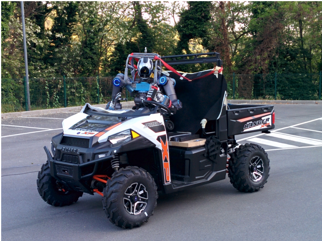
Figure 5.1: The Walk-Man robot in a driving configuration.
