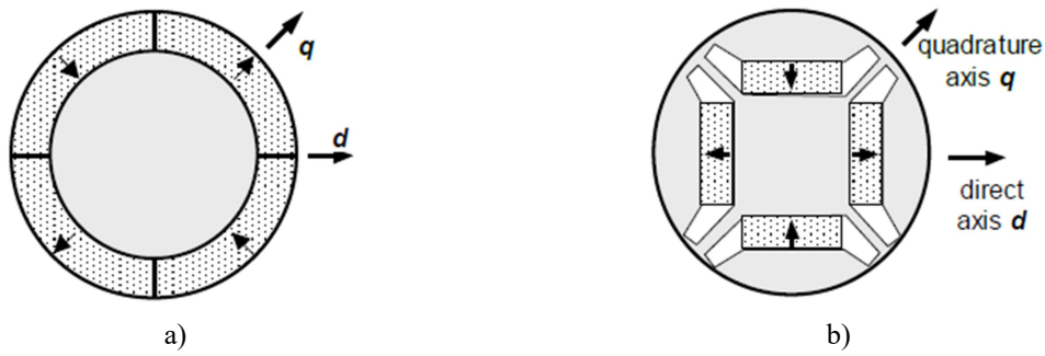
Figure 18 a) SPSM Isotropic b) IPMSM Anisotropic [4]
