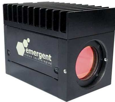
Figure 3.6: The Emergent Vision Technologies HT-12000 10 GigE Camera
