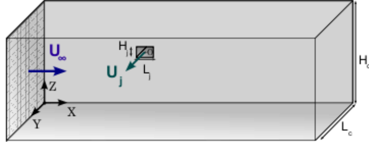
Figure 2.18: Schematization of the Transat test section. Fougairolle [? ].
