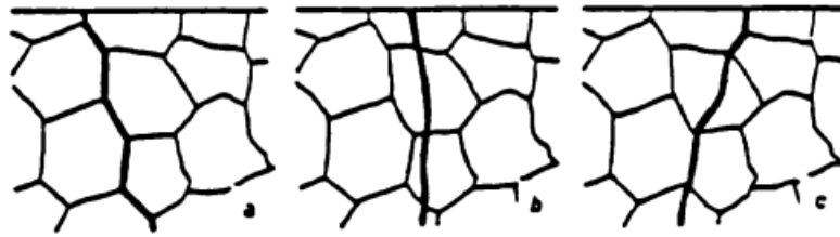
Figure 1.10: Scheme of different cracks propagations within the crystalline lattice: a) Transcrystalline regime ; b) Intracrystalline regime ; c) Mixed behaviour. Merola and Biggio (1988) [? ]
