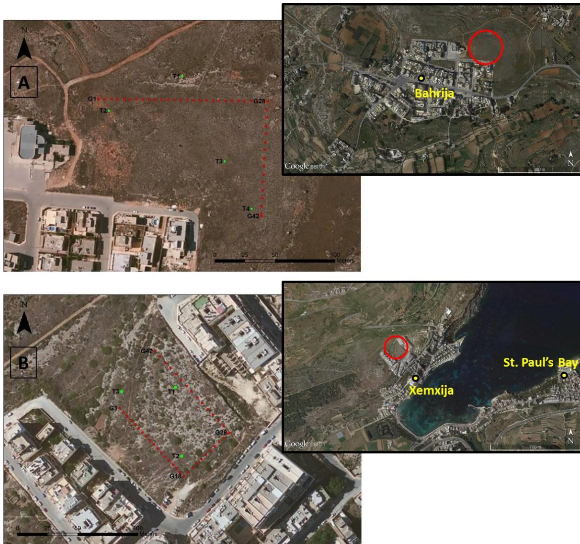
Fig. 5.3 - Passive seismic survey at Bahrija (A) and Xemxija (B). The red circles in the sketch indicate the position of the investigated sites respect to the urban areas. The red dots show the position of each geophone of the seismic arrays while the Gxx at the corners of the two array configurations indicate the number of the geophone found in that corner. The green points show the location of the single-station acquisitions (modified from Farrugia et al. , 2016).
