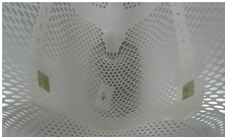
Figure 5.5: An example of in vivo measurement setup with EBT3 in tomotherapy using a thermoplastic mask.
