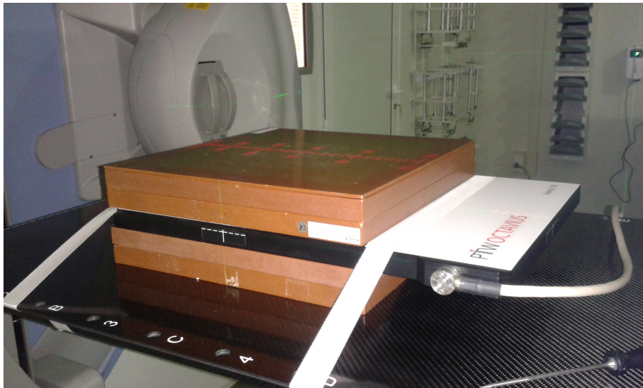
Figure 4.2: Measurement setup during validation measurements performed with PTW 2D-Array 729 at Linac.
