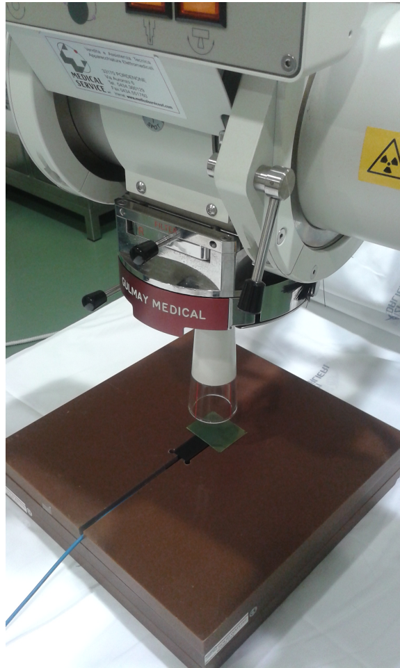
Figure 3.1: Experimental setup used during the preliminary measurements and the calibration in Plesio therapy. For the measurements made before the calibration, the dose was read by a plan parallel ionizing chamber with and without the film piece. When present, the film sample was located at direct contact with the chamber and with a circular applicator (5 cm diameter) during the measurements.
