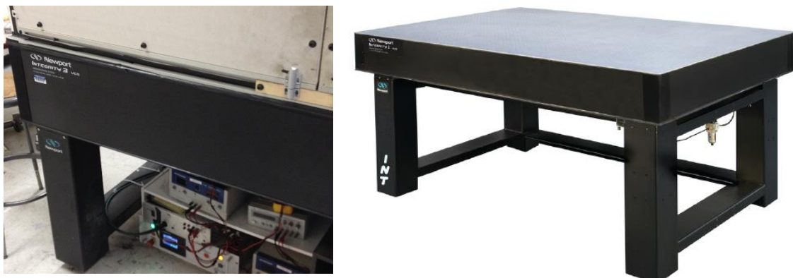
Figure 2.2: Newport optical table with precision tuned damper supporting the box setup [46].
