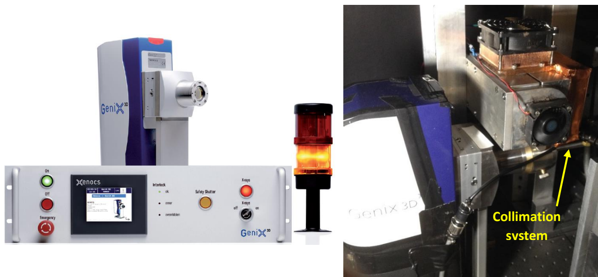
Figure 2.3: Genix 3D monochromatic source system (left) and inside the setup with vacuum-enhanced collimation (right) [47].
