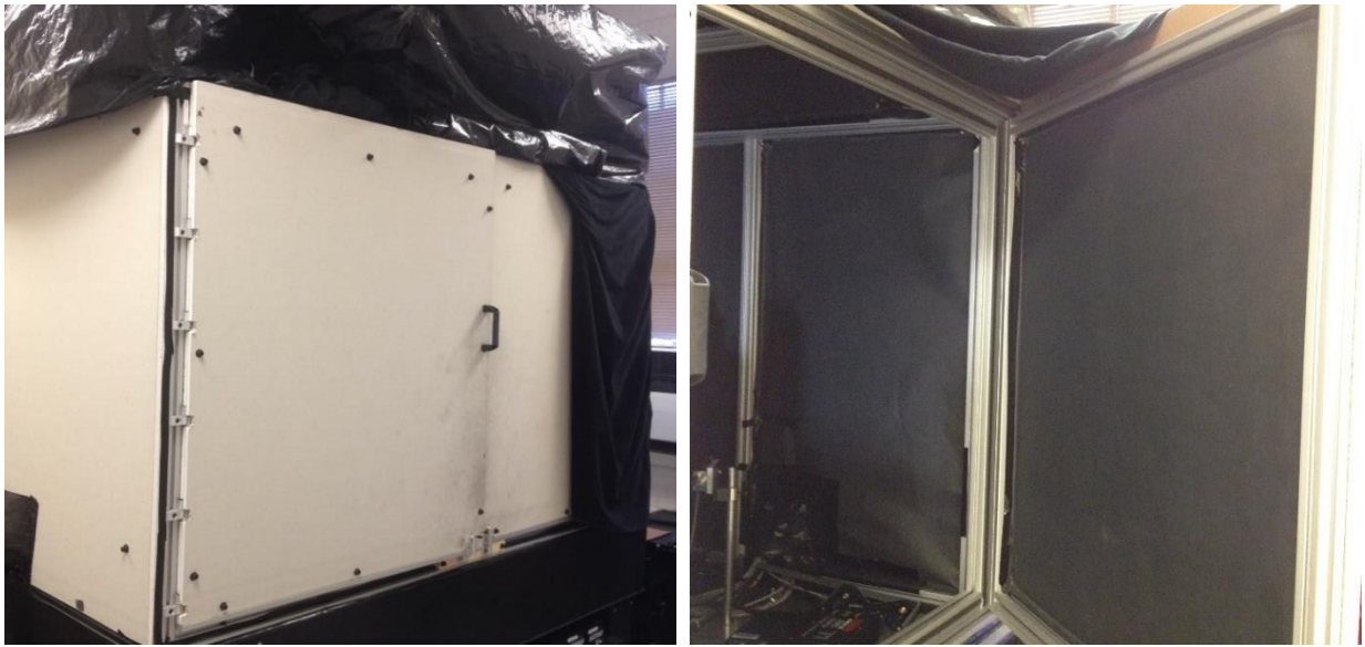
Figure 2.1: Box structure containing the XFCT/XLCT system (left) and blackened internal walls (right).
