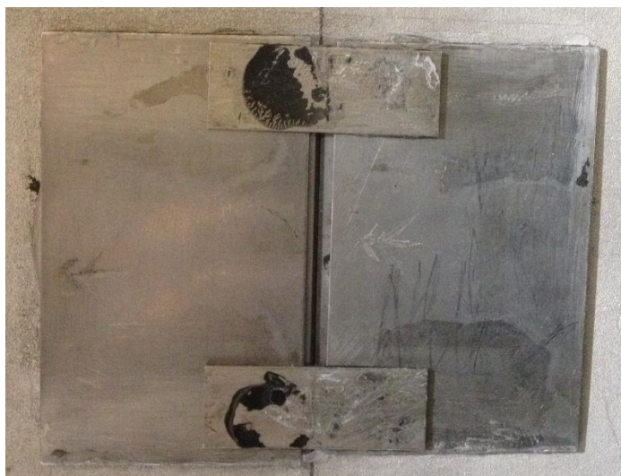
Figure 4.16: Picture of the 100 \mu\text{m} -single slit aperture used in the XFCT imaging study [62].
