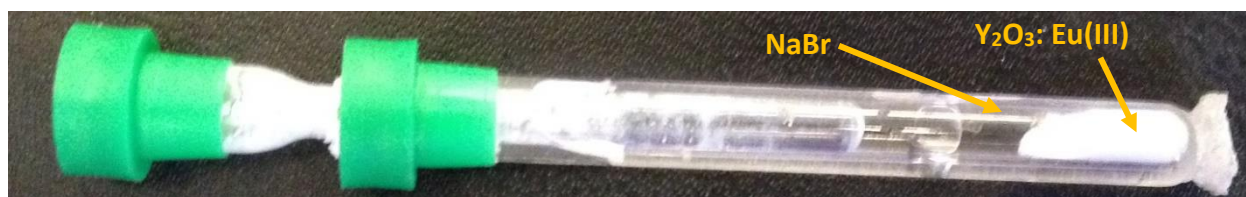
Figure 4.17: Glass double tube filled with Y_2O_3:Eu(III) nanoparticles in powder form (inside) and NaBr in water solution (outside) [62].
