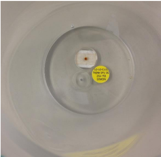
Figure 4.15: sources of ^{241}\text{Am} and ^{152}\text{Eu} used for QA
