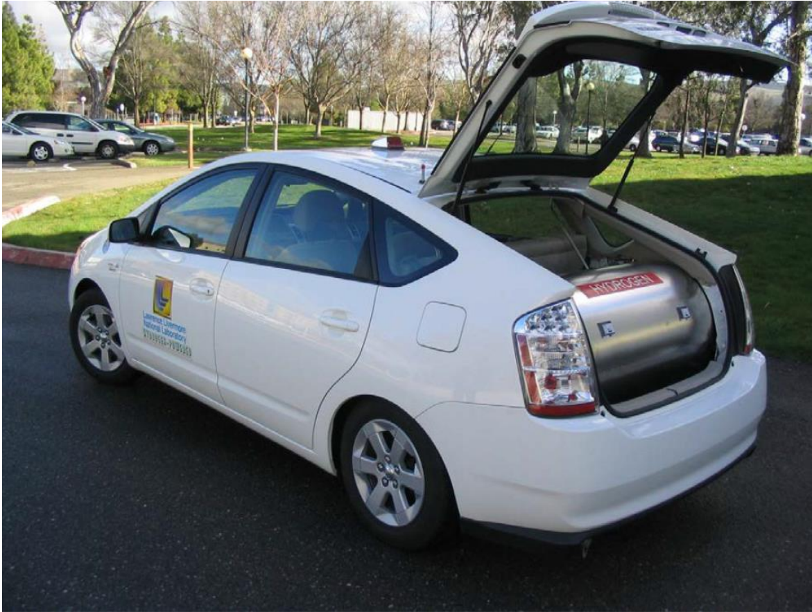
FIGURE 19 CRYOGENIC PRESSURE VESSEL INSTALLED ONBOARD A HYDROGEN-FUELED TOYOTA PRIUS EXPERIMENTAL VEHICLE
