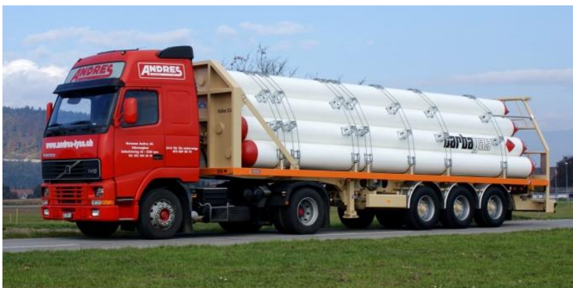
FIGURE 39 TRUCK WITH TUBE TRAILER FOR COMPRESSED HYDROGEN DELIVERY
