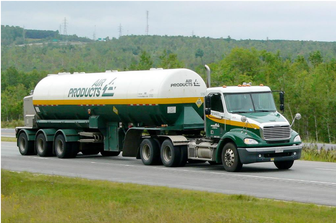
FIGURE 35 CRYOGENIC LIQUID HYDROGEN TANKER TRUCK
