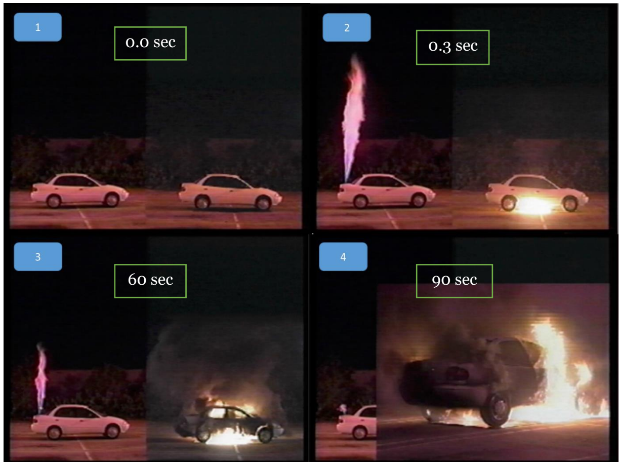
FIGURE 1 HYDROGEN POWERED VEHICLE ON THE LEFT. GASOLINE POWERED VEHICLE ON THE RIGHT. TIME-SEQUENCE FUEL LEAKAGE.
