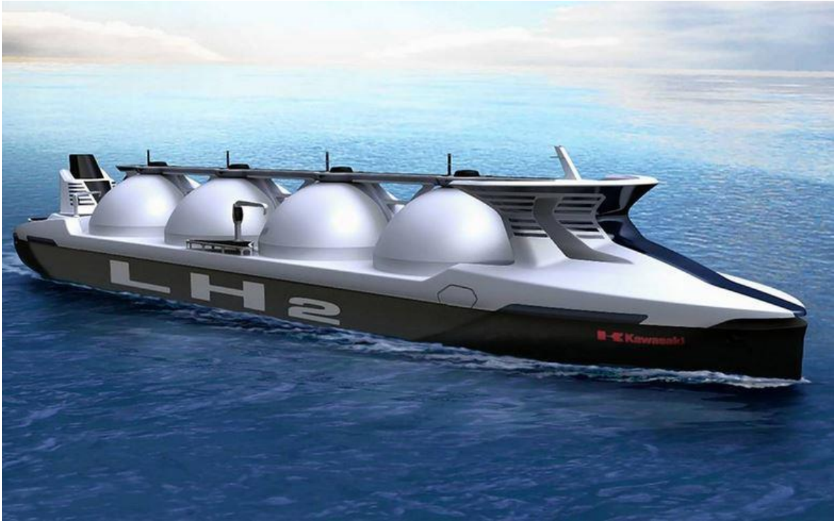
FIGURE 37 CONCEPTUAL DESIGN OF 160000 m 3 LH2 CARRIER SHIP
