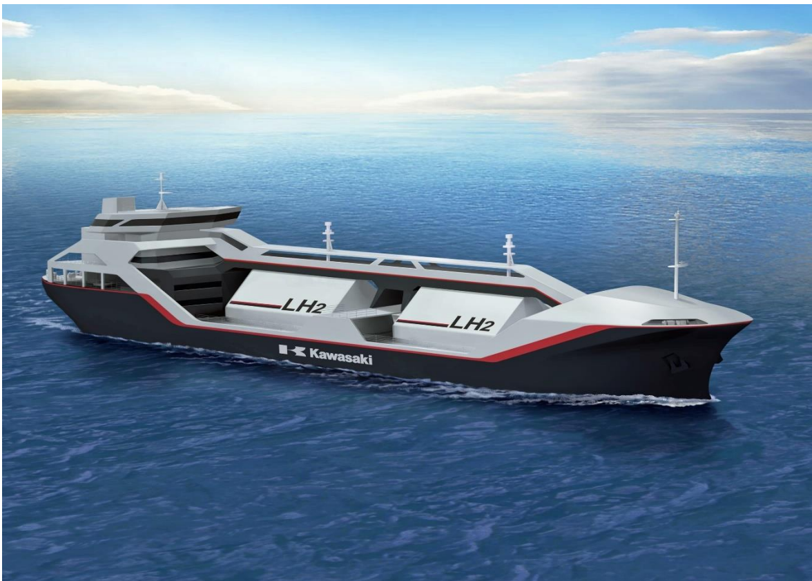
FIGURE 38 CONCEPTUAL DESIGN OF 2500 m 3 LH2 CARRIER SHIP
