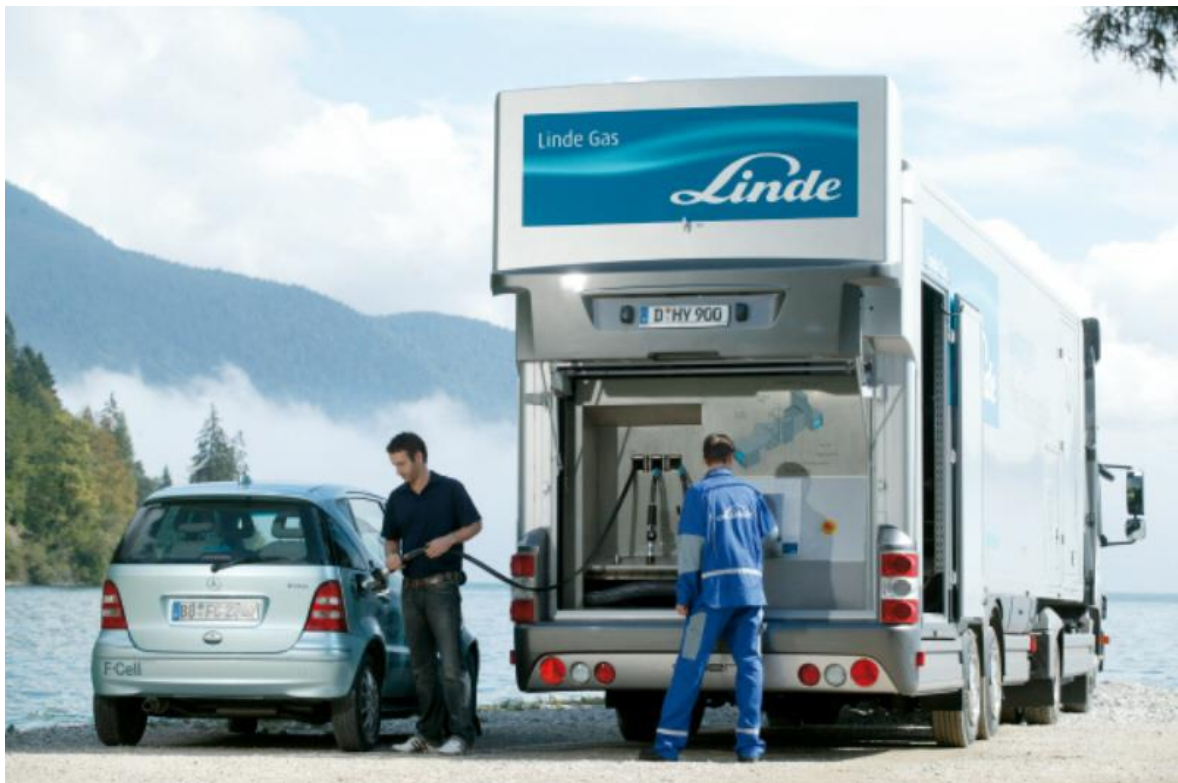
FIGURE 46 MOBILE HYDROGEN REFUELING STATION
