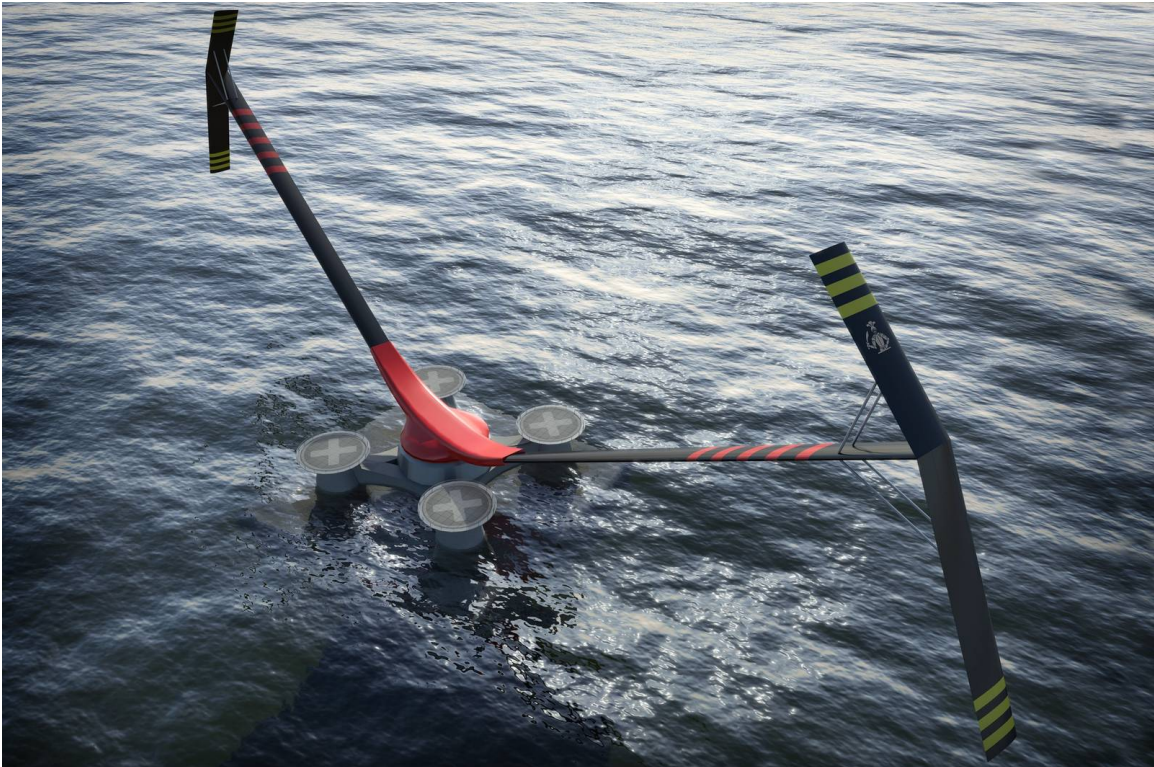
Figure 1-8: The aerogenerator X, an example of new VAWT design for floating applications.
