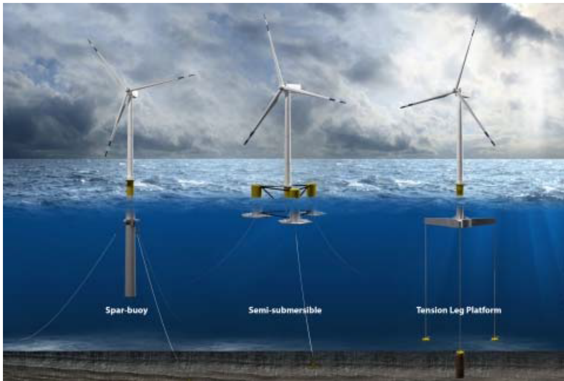
Figure 1-5: Floating wind foundation typologies (DNV-GL, 2014).
