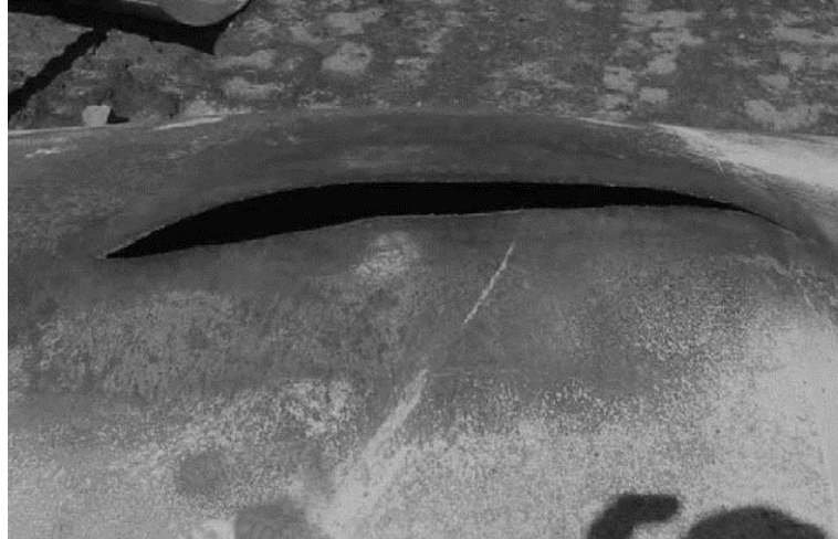
Figure 3.11– Tank failure, test 04-03 [Birk et al. 2006]
