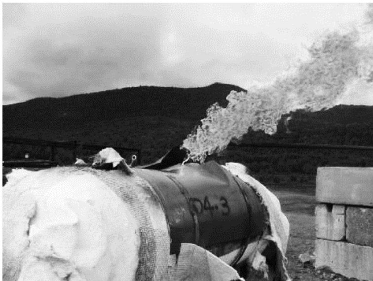
Figure 3.10 – Test 04-03 tank after rupture. The steel jacket split open at the top tack weld. [Birk et al. 2006]
