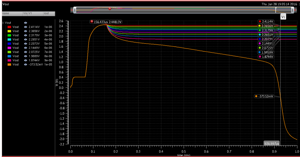
Figure 5.14: 4 MHz transient simulation of the old converter D.
