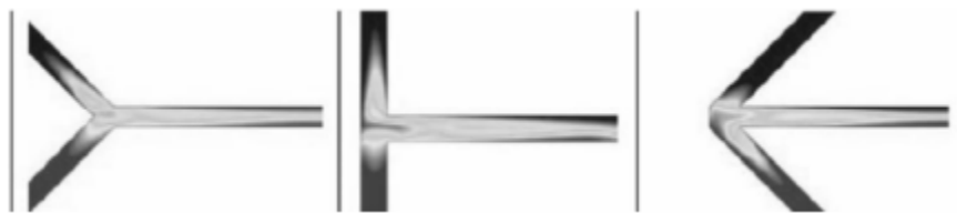
Figure 1.2.5: Micromixers at “Y” intersection, “T” intersection, and arrowhead intersection
