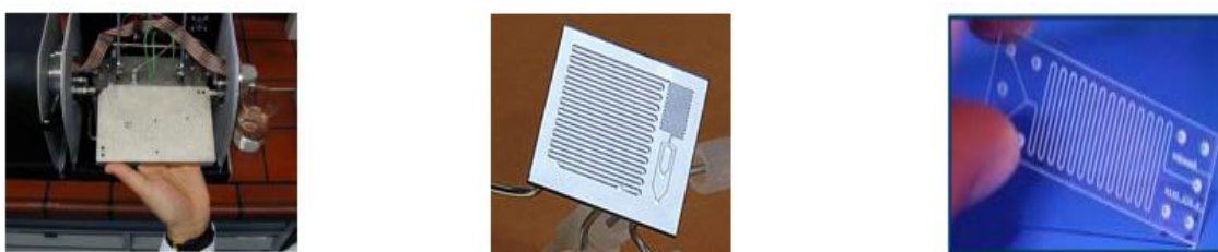
Figure 1.2.2: a) polymer, b) metallic and c) glass Micro-flow reactors
