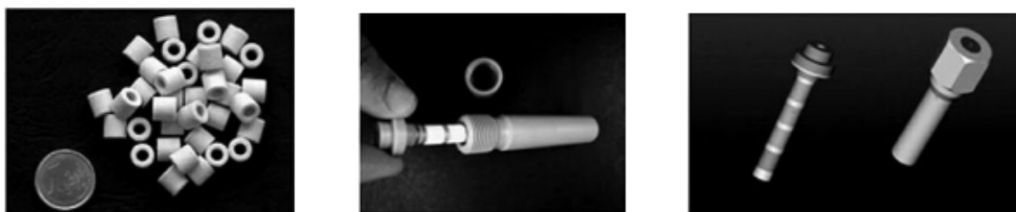
Figure 2.3.3.2: Raschig rings aligned on a perforated tube, within a PEEK polymer casing.
