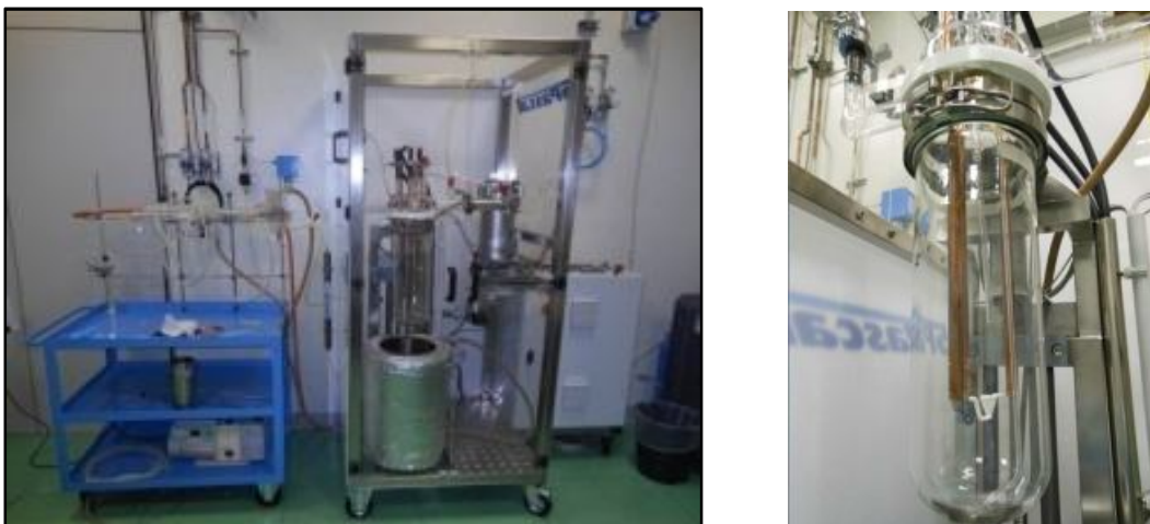
Figure 2.1.6: a) MVS apparatus for the synthesis of mono- and bimetallic nanoparticles (Pd, Au, Pt, Ni, Rh, Co, Cu) b) Glass reactor equipped with joule effect heating for vaporization one or two metals simultaneously
