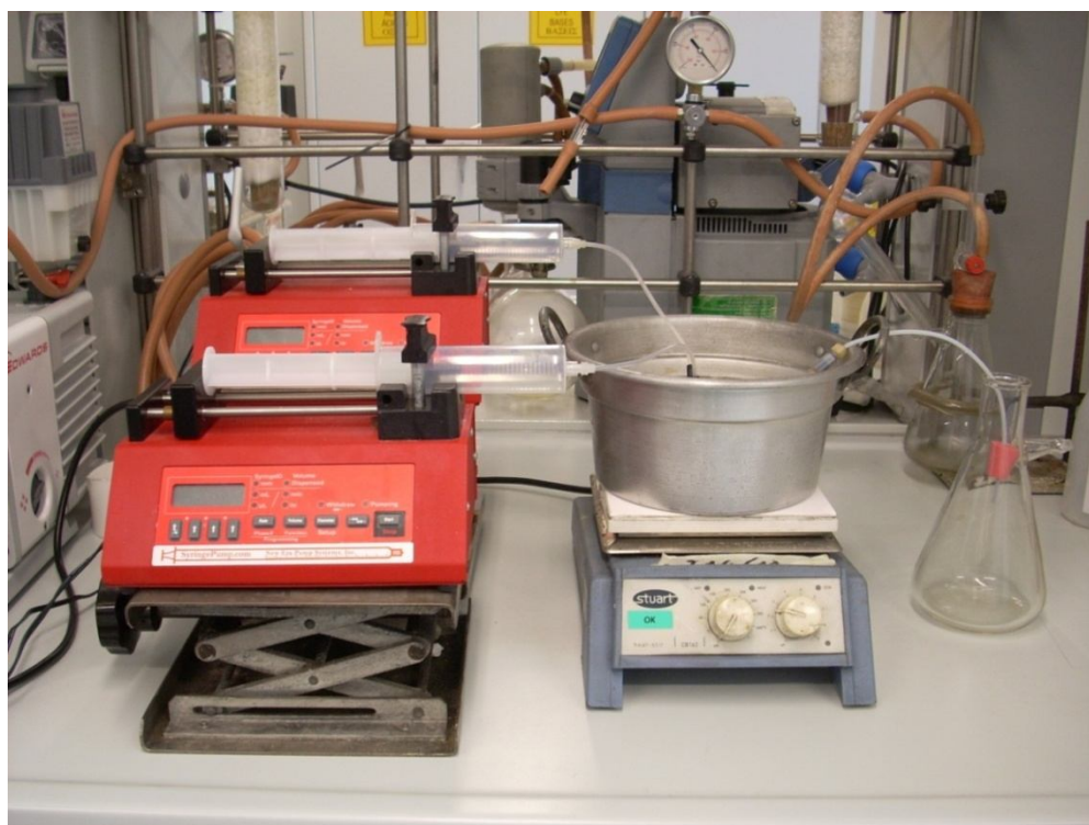
Figure 2.2.5: Our simple and cheap continuous flow system
