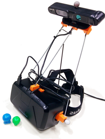
Figure 3.2: The visualization system: Oculus Rift DK2 and PrimeSense Carmine 1.09
