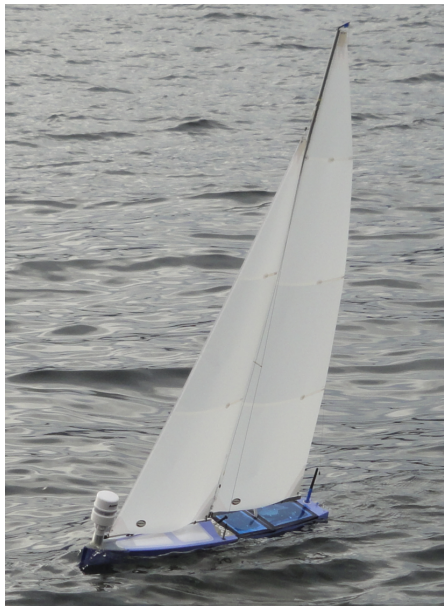
Figure 1.3: AEOLUS, the autonomous sailing model boat.
