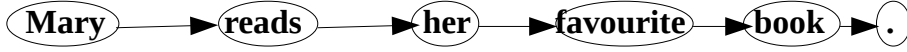
Figure 5.1: A graph neural network for a monolingual language model. Each word corresponds to vertex which shares a (directed) edge only with the vertexes of the adjacent words.
