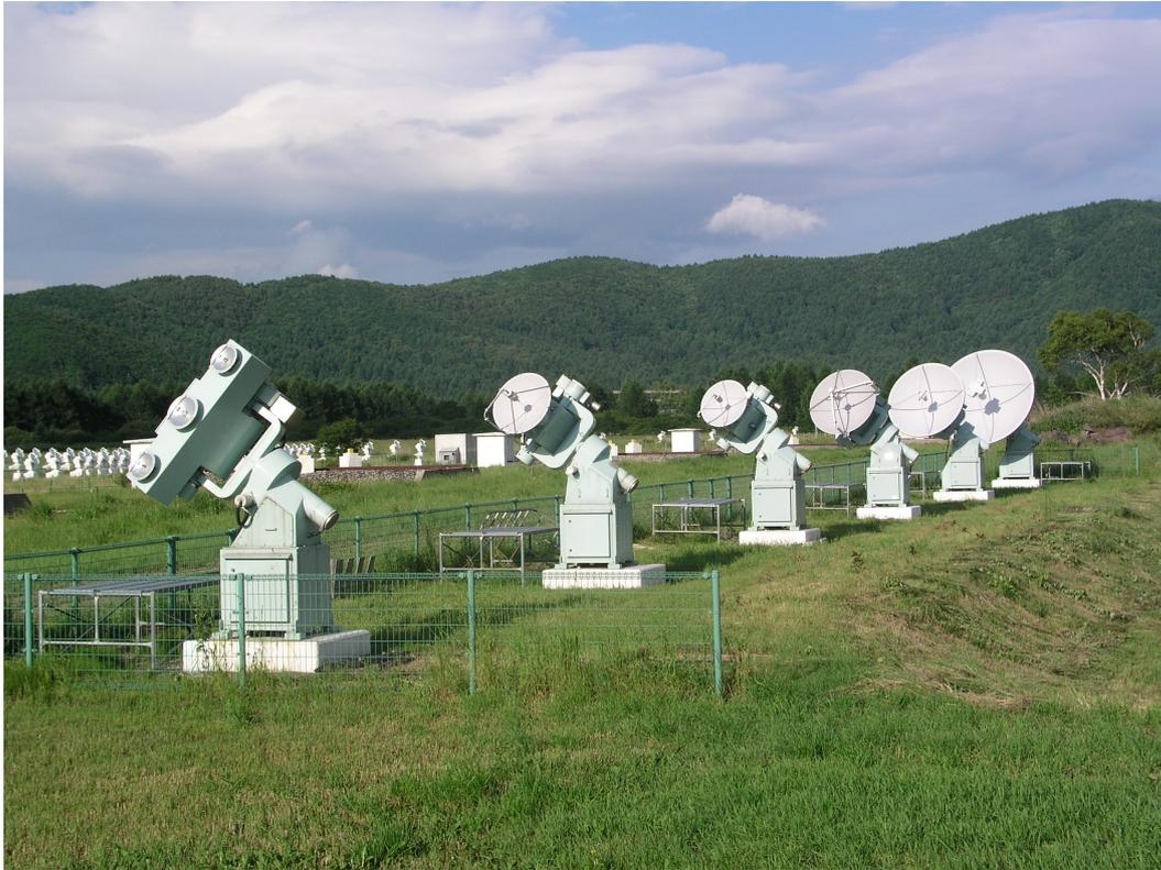
Figure 4.1: Nobeyama Radio Polarimeter, image from [http://www.nro.nao.ac.jp/en/gallery/images/rp\\_002.jpg](http://www.nro.nao.ac.jp/en/gallery/images/rp_002.jpg). On the left there's the single mount with three antennas, where the central one is for the 35 GHz observations while the other two are for the 80 GHz observations; the other antennas, from left to right, are for 17, 9.4, 3.75, 2 and 1 GHz observations.
