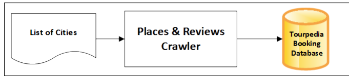
Figure 3.23: Logical architecture of Booking.com Data Extractor
