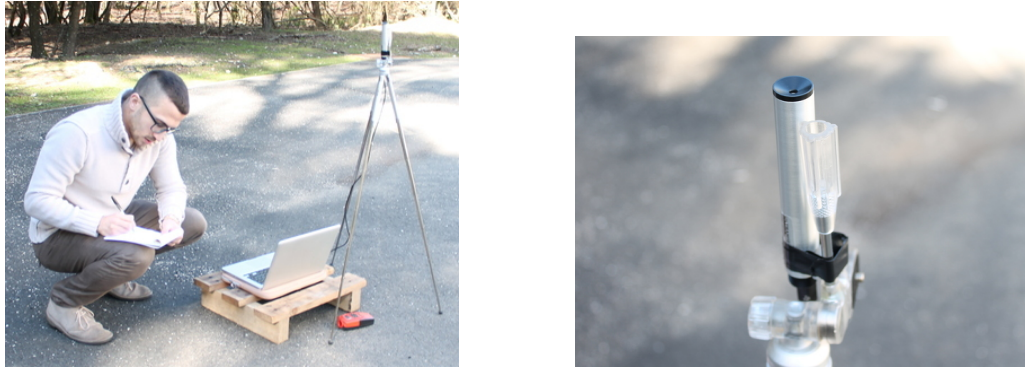
FIGURE 4.7: Sensor Configuration: the microphone is positioned on a tripod and connected to a PC via USB
