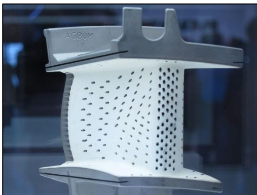
Figure 7-5 NGV after the repair process (Cleynen, 2013).
