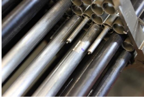
Figure 21: TCs positioning and fixing
