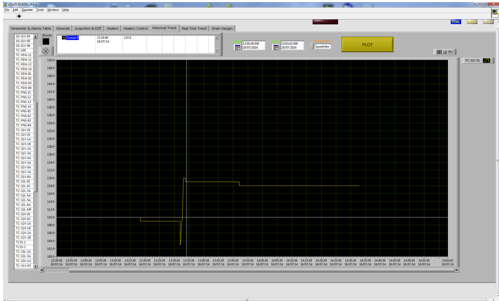
Figure 4.26 – pressure time trend during the pressure test of LIFUS5/Mod2 facility with LEADER test section
