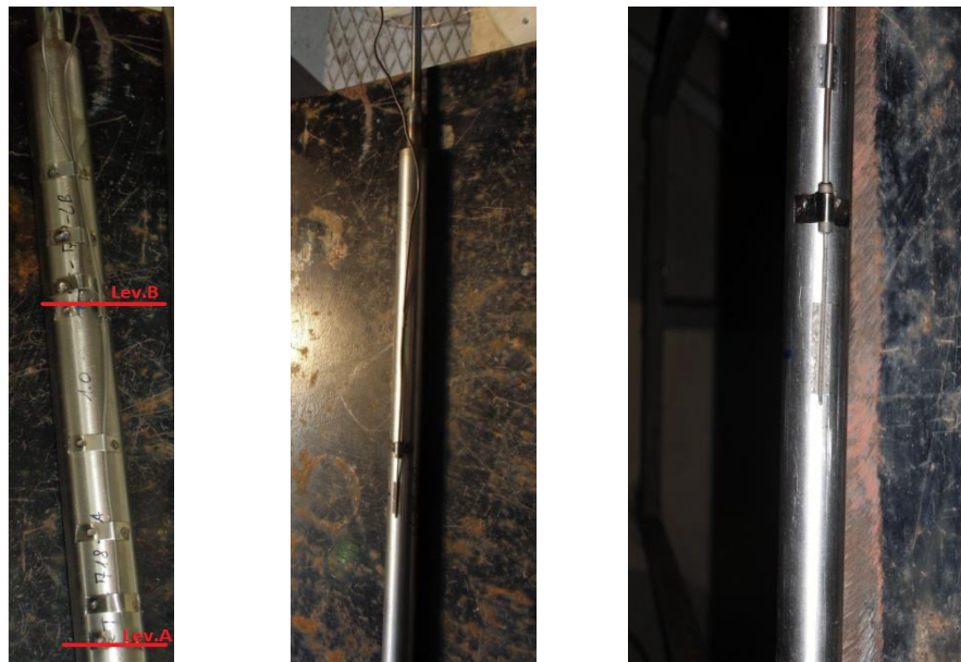
Figure 4.17 – view of thermocouples (left) and strain gages (center and right)
