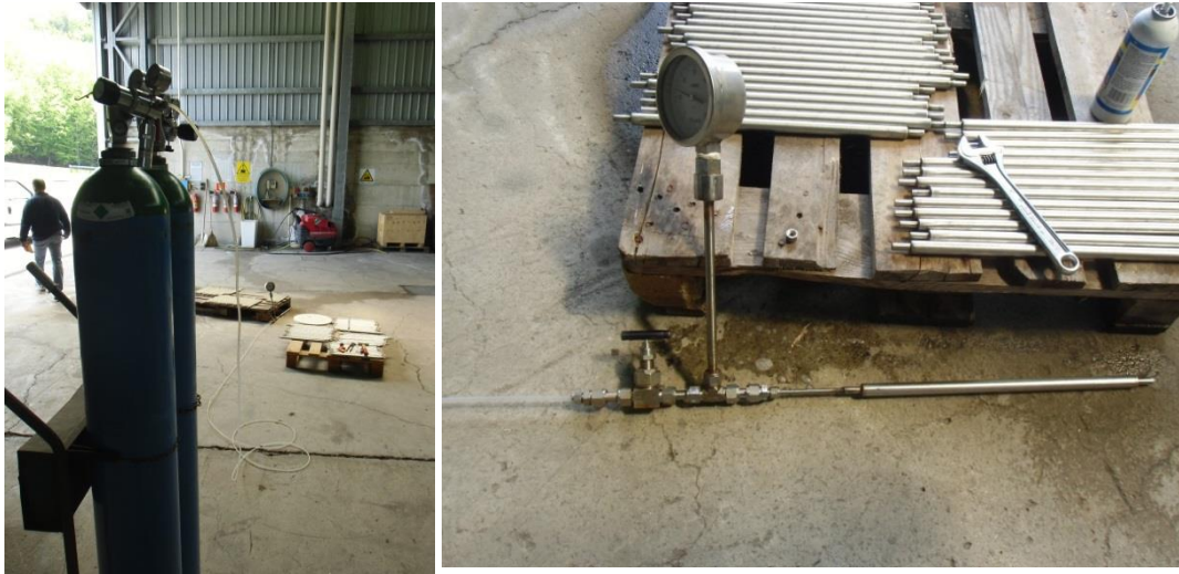
Figure 4.18 – pressure test of pressurized tubes
