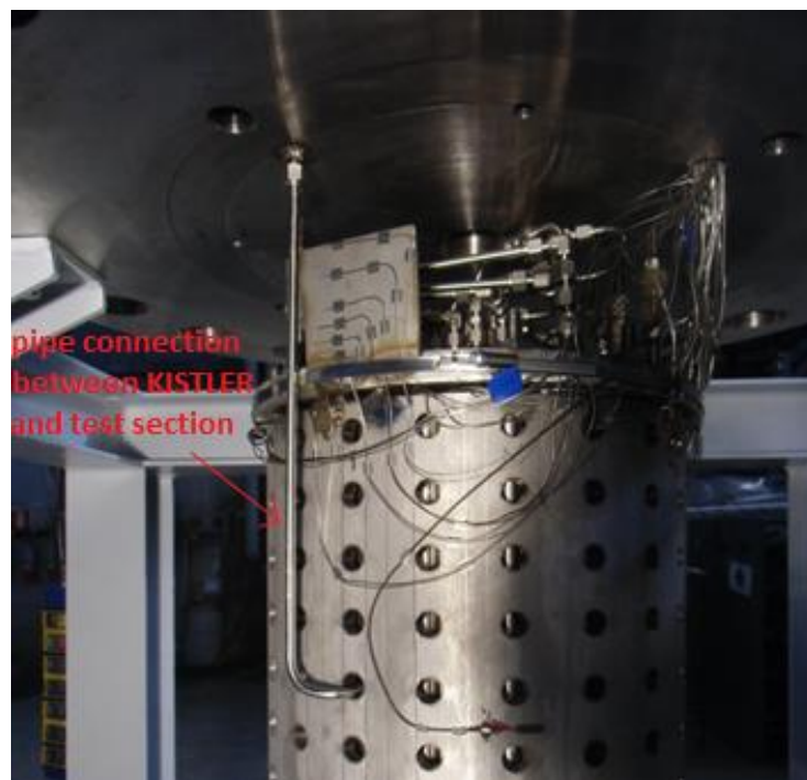
Figure 4.22 – pipe connection between LEADER test section and KISTLER PT on S1 top flange
