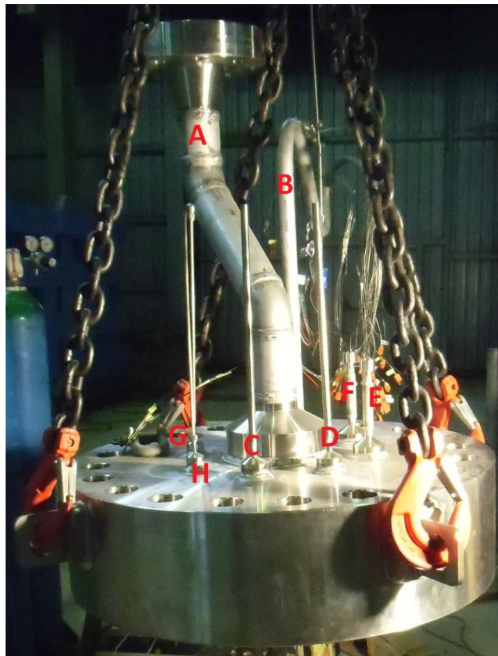
Figure 4.6 – view of S1 flange penetrations
