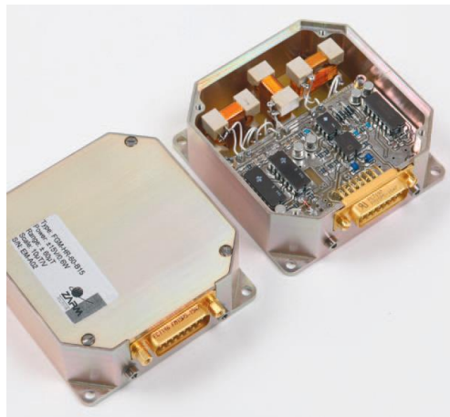
Figure 9.9: AMR ZARM digital magnetometer.
