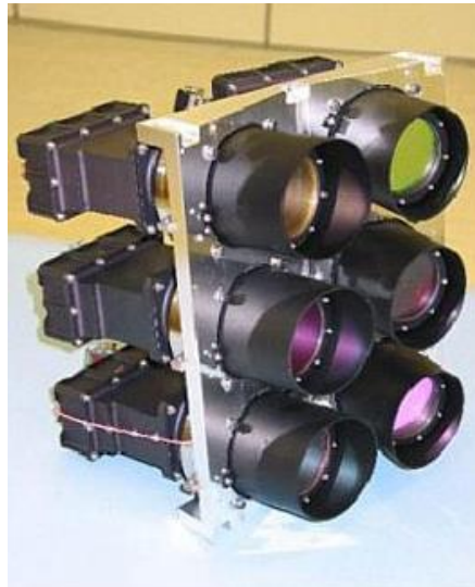
Figure 1.2: The DMC SLIM-6-22 12 kg instrument.
