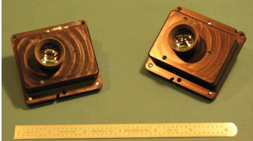
Figure 9.10: ST-16 Sinclair star trackers.
