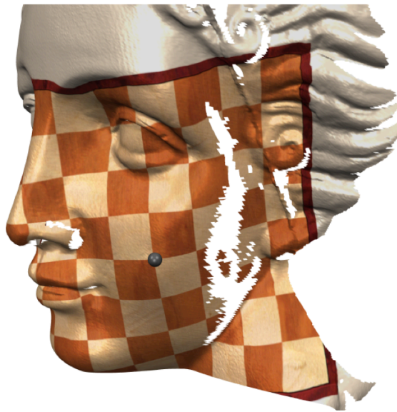
Figure 1.8: Texture mapping on a FACE model containing holes due to occlusion effects.
