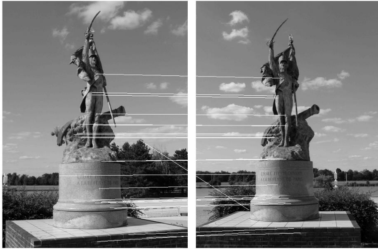
Figure 13: Correspondences between features in the left image and in the right one.
