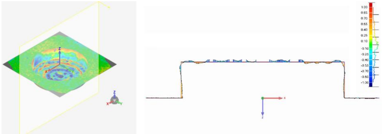
Figure 5.15. Deviation of the bottom surface of the grooved cylinder from an ideal planar surface.
