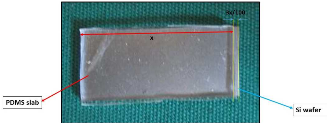
Figure 2.6: PDMS slab with its of the original size on a silicon wafer having a length that is 103% strain of the PDMS slab length.
