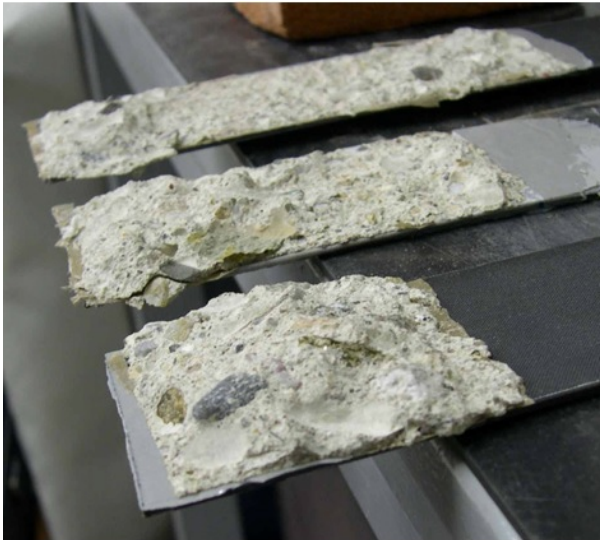
Figure 2.14: Bulbs at FRP free end for different lengths of the reinforcement [34].
