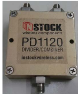
Fig. 3.6 Power Divider 3 dB (PD1120 IN-Stock) used in the measurement setup.
