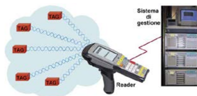
Fig. 1.4 A management system control for RFID UHF reader
