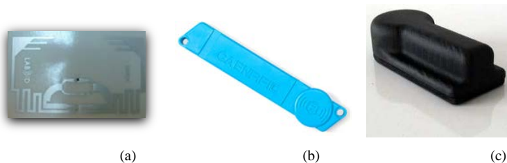
Fig. 1.5 Example of UHF tags (Ultra High Frequency): passive, Lab-Id UH414 (a), semi-passive, CAEN RFID A927Z (b), active IDN-ABG245AT (c).
