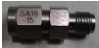
Fig. 3.16 Attenuator (SA18 SM-15: Electronics) with Insertion Loss of 15 dB used in the measurement setup.
