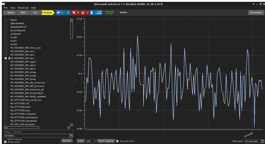
Figure 2.9: Ground Station: Plotting of received sensor data
