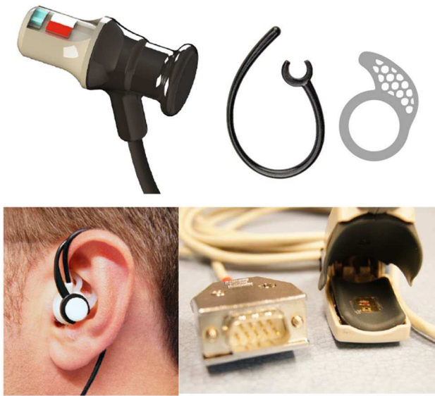
Fig. 2 A 3D sketch of ear canal PPG sensor, photograph of an assembled ear canal PPG sensor placed inside the right ear of a volunteer and a photograph of the finger sensor
