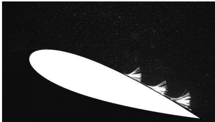
Figure 4: Image of the field of view for a hairy flap configuration (No. 6) at constant angle of attack \alpha=17.5^\circ .
