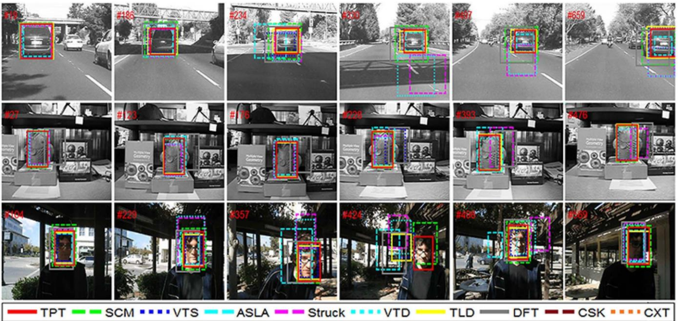
Fig. 9. From top to bottom are representative results on sequences Car4 , Fish , and Trellis , where objects suffer from significant illumination variations.
