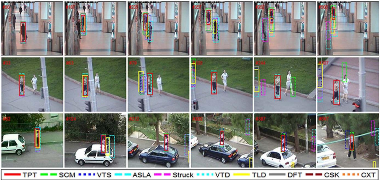
Fig. 8. From top to bottom are representative results of trackers on sequences Walking2 , Jogging1 , and Woman , where objects are heavily occluded.
