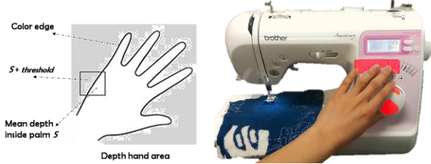
Figure 3. Touch detection based on contour searching in depth (left). Detected touch areas are shown in red (right).
