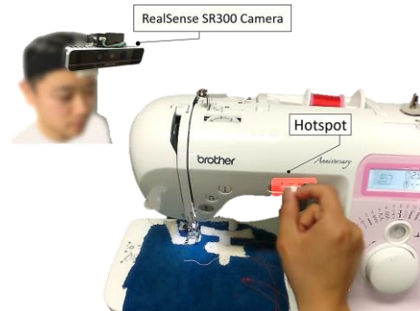
Figure 1. Machine operation experimental environment. Head-mounted RGB-D camera (top-left) records experiences while users are operating a sewing machine.
