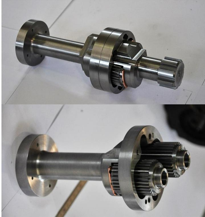
Figure 31 Redesigned replica of the planetary transmission of the IDG
