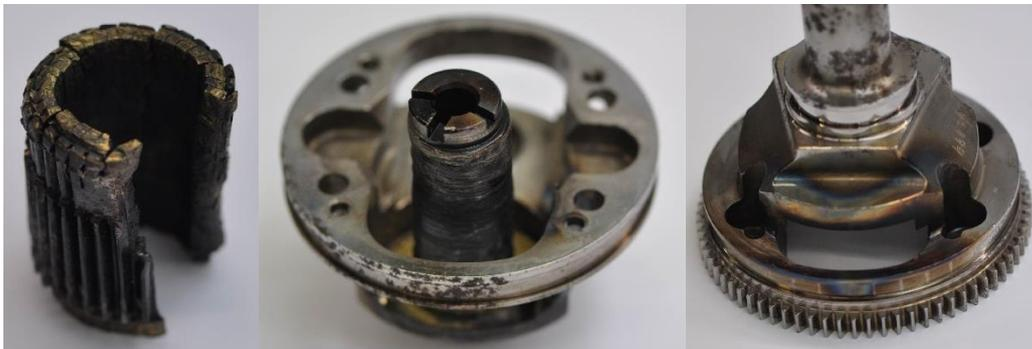
Figure 4 Example of damage of adjacent components (left: planetary gear  $\text{Ø}=37\text{mm}$ , centre: carrier shaft  $\text{Ø}=94\text{mm}$  and bearing shaft  $\text{Ø}=24\text{mm}$ , left: carrier shaft 2  $\text{Ø}=94\text{mm}$ )
