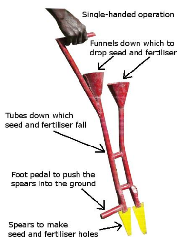
Fig. 2: Design of the Spear Planter
