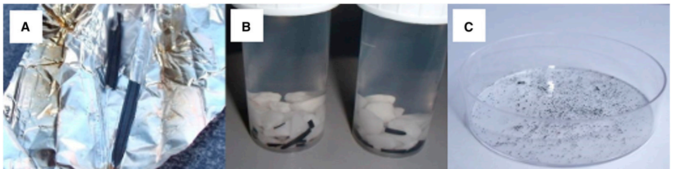
Fig. 1. Charcoal samples, as removed from furnace (A), prior to simulated transport with water and gravel (B), and dispersed on a Petri dish prior to imaging (C).
