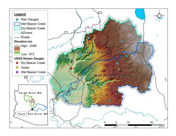
**Fig. 1.** Beaver Creek watershed location within the Verde River in central Arizona (inset). Watershed representation through a 30 m Digital Elevation Model (DEM) and the locations of stream gauges, rain gauges and sub-watershed boundaries (Wet and Dry Beaver Creek).
