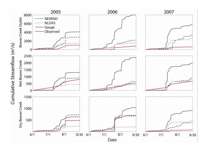
**Fig. 6.** Simulated and observed cumulative streamflow (June 1 to September 30) for the three summer periods at the three stream gauges from the Gauge, NEXRAD and NLDAS products.
