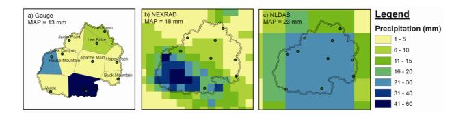
**Fig. 4.** Spatial distribution of total event precipitation on July 28, 2007 from Gauge, NEXRAD and NLDAS products, with the watershed boundary and mean areal precipitation (MAP) shown.
