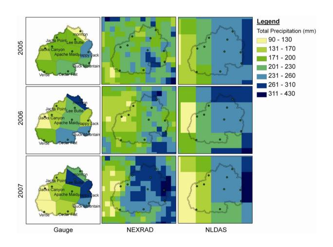
**Fig. 3.** Spatial distribution of total precipitation for three summer periods from Gauge, NEXRAD (4 km) and NLDAS (12 km) products over Beaver Creek (with watershed boundary shown).
