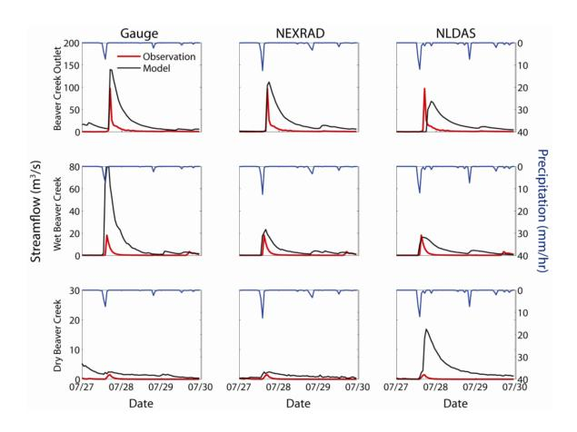
**Fig. 5.** Simulated and observed streamflow (July 27 to 30, 2007) at the three stream gauges from the Gauge, NEXRAD and NLDAS products with the spatially-averaged precipitation shown.
