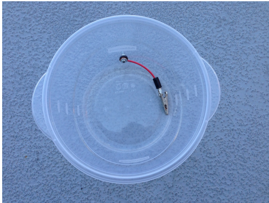
Figure 4.3.1 Container for Dielectric Oil
