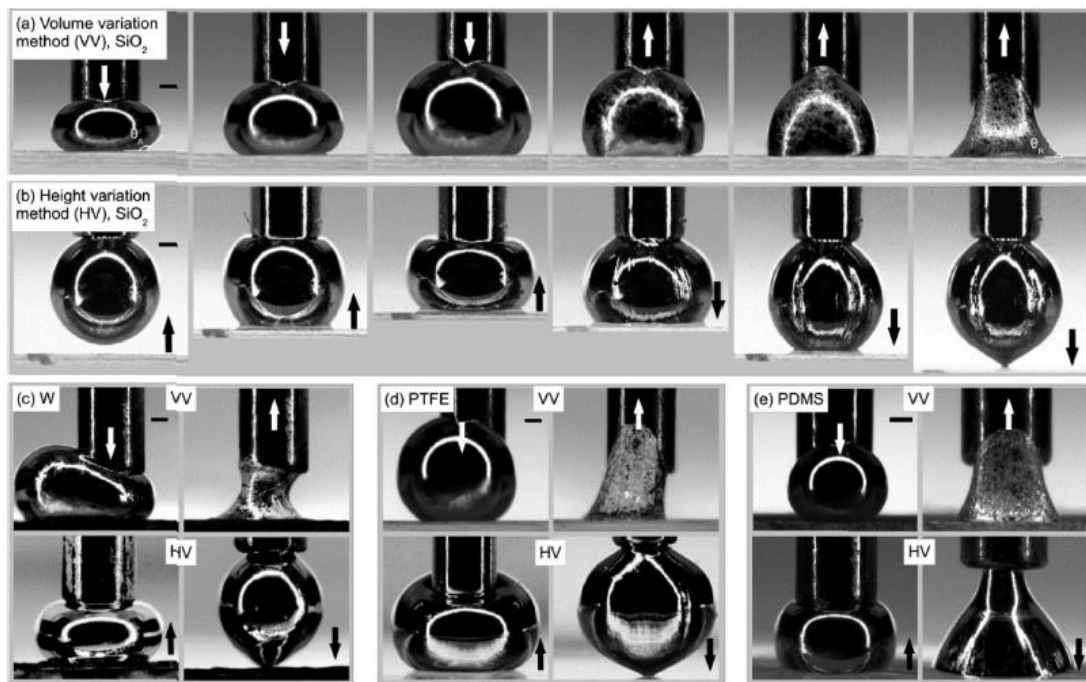
Figure 2.5 Optical images of advancing and receding contact angles of GaInSn on (a, b) glass, (c) tungsten, (d) PTFE, and (e) PDMS surfaces measured using volume (VV) and substrate height variation (HV) methods in air at about 98 kPa. The scale bar corresponds to 230 \mu\text{m} .
