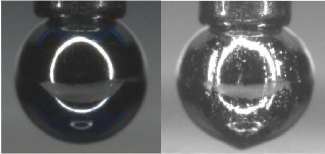
Figure A GaInSn drop before and after height variation test. The perimeter of the drops is nearly identical before and after the test.
