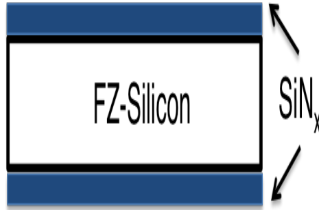
Fig. 6.1: Test structure to measure minority carrier lifetime ( \tau_{\text{eff}} )
