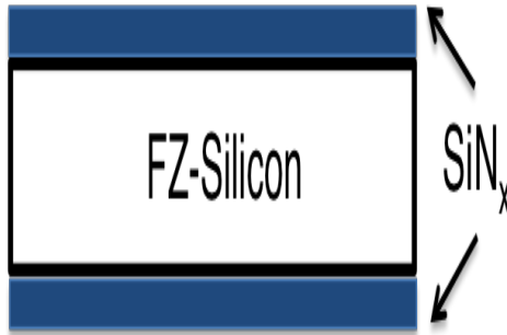
Fig. 4.10: Test structure for measuring effective carrier lifetime and surface recombination velocity
