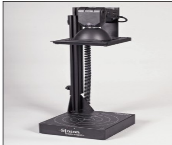
Fig. 4.11: Sinton instruments WCT-120 wafer lifetime tester
