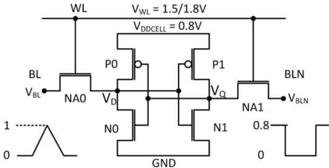
**Figure 2.1** Singled ended test circuit showing different power supply voltages to sample SRAM cell switch points.
