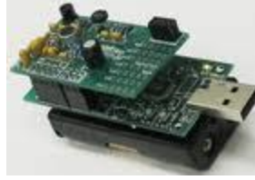
Figure 3 Telos revision B with detachable sensors
