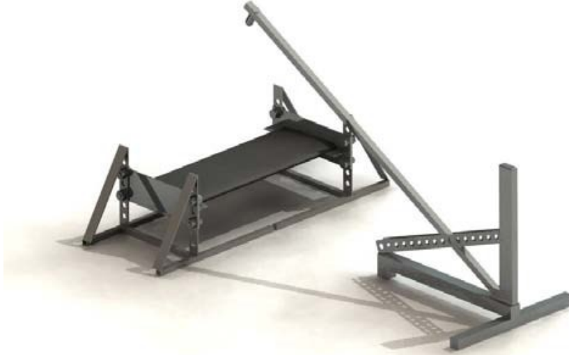
Figure 4.9. Experimental apparatus setup for airfoil impact.
