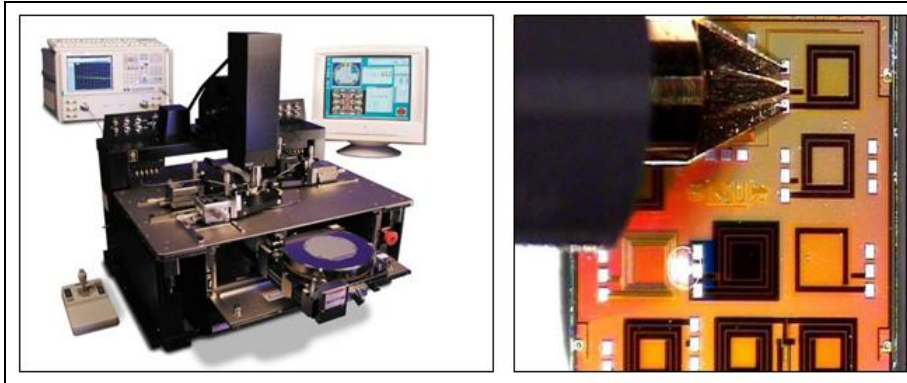
Figure 40: Test & Characterization of Spiral Inductor
