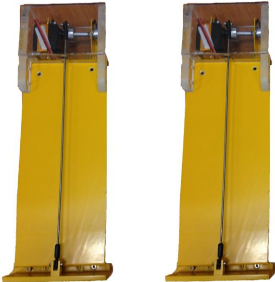
Figure 3: Electrically activated model scale T-Foil.
