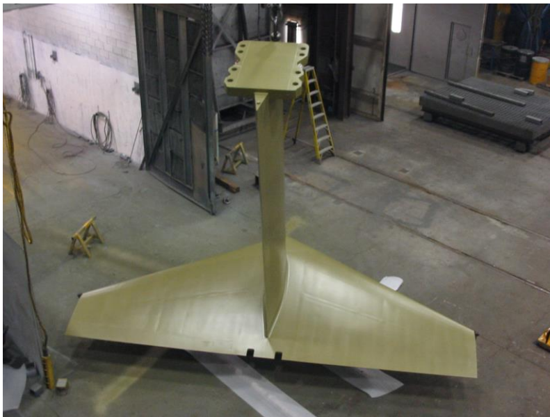
Figure 2: Full scale T-Foil prior to installation on a 112 m INCAT Tasmania high-speed wave-piercing catamaran [2].
