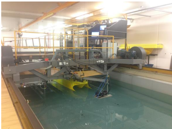
Figure 8: The catamaran model attached to the moving carriage.
