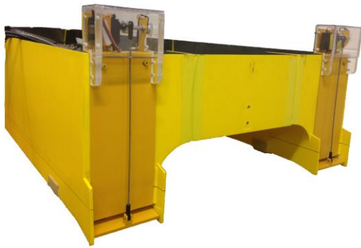
Figure 7: Stern tabs installed at the aft end of the model.
