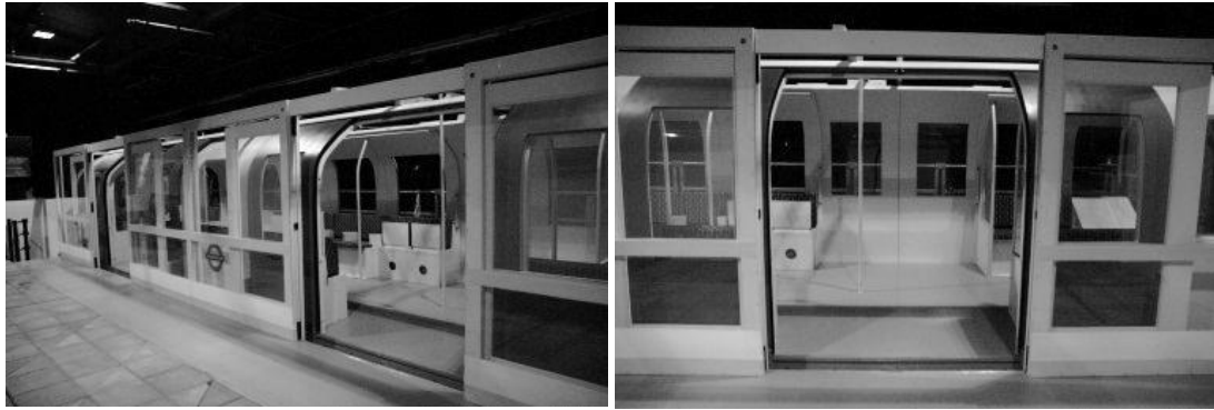
Figure 1: Sample images of the mock-up train carriage at the PAMLEA facility with Platform Edge Doors (PEDs)
