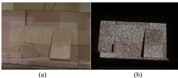
Figure 2. Random dot texture projection using a data projector. (a) with ambient illumination (b) with projector only.
