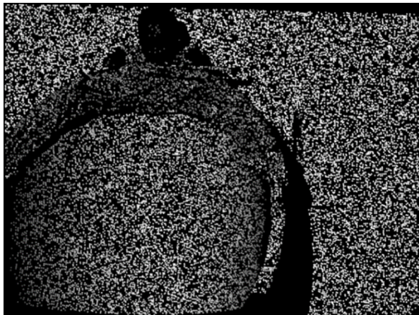
Figure 8 Simulated random dot pattern, generated from 35,000 LIDAR points mapped to image coordinates. Each point is a 5 pixel white circle and a Gaussian convolution was applied to the image.
