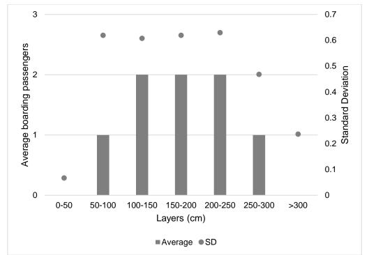
Figure 5. Average location of passengers on the platform waiting to board the train at GPK in the AM and PM peak hours
