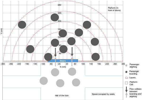
Figure 1. Model divided in concentric layers of 50 cm each to measure behaviour and interaction on platforms formed of 40 cm square cells
