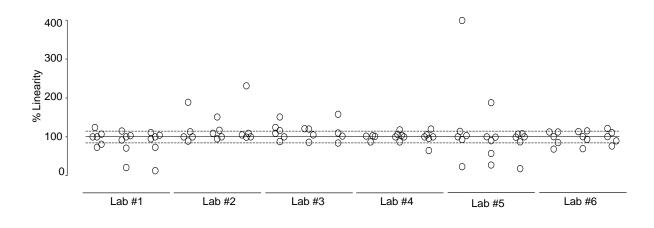
**Figure 2. Linearity of dilution.** The data showed that dilution of linearity was largely within the predefined range of 85%-115%. The graph shows % linearity for three samples per lab. The continuous line indicates 100% linearity and two dotted lines indicate lower (85%) and upper (115%) pre-defined ranges respectively. The "hook effect" was not observed in any of the laboratories (data not shown).
